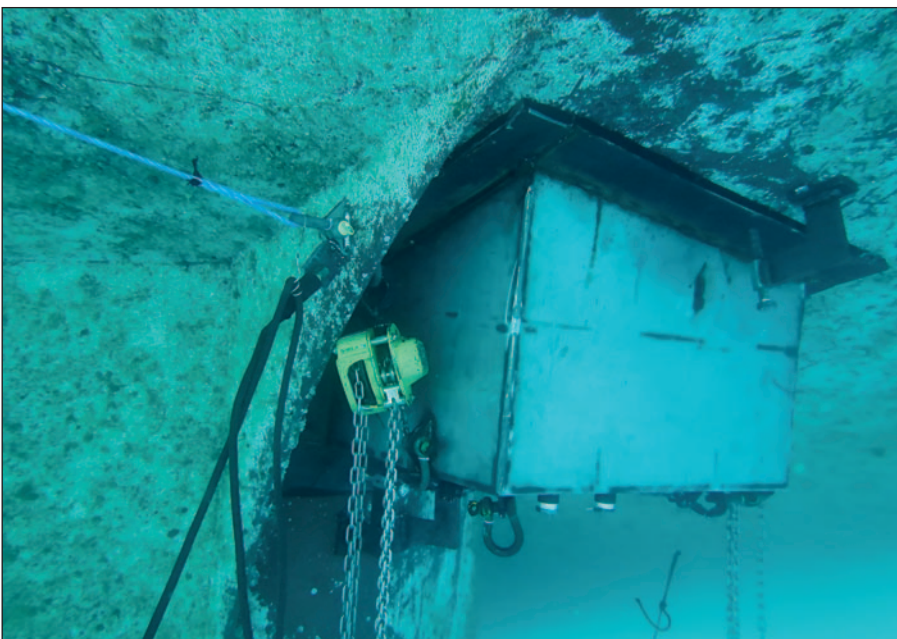
Tailor-made cofferdam on drill ship in Palermo.
