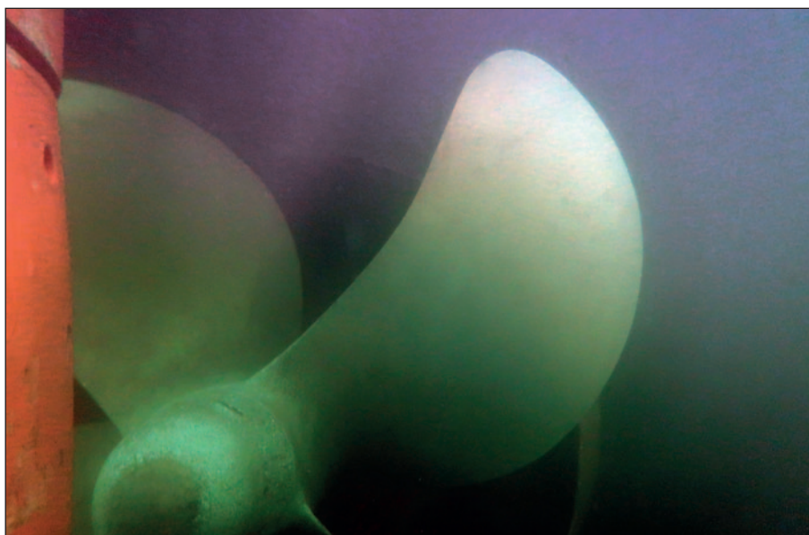
Propeller blade after straightening.
