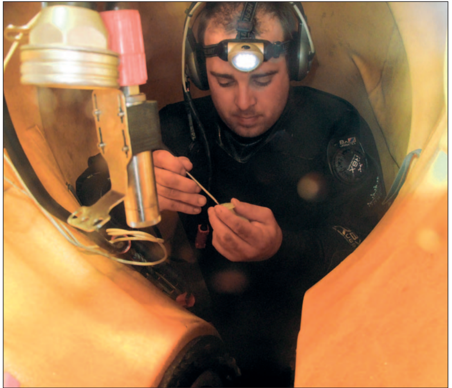
Toon Joos, Chief Diver, working in dry conditions on a stern tube seal inside a flexible mobdock, a Hydrex development for safe in-water stern tube seal operations.
