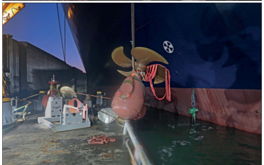
Old thruster unit brought to the surface.
