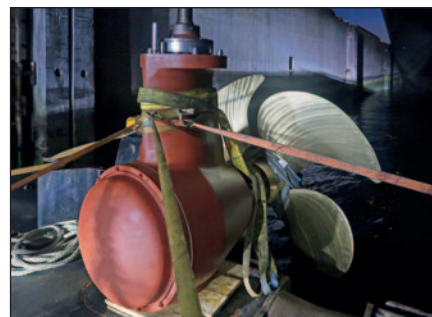
Bow thruster replacement on roro ship in Rotterdam 4-6
