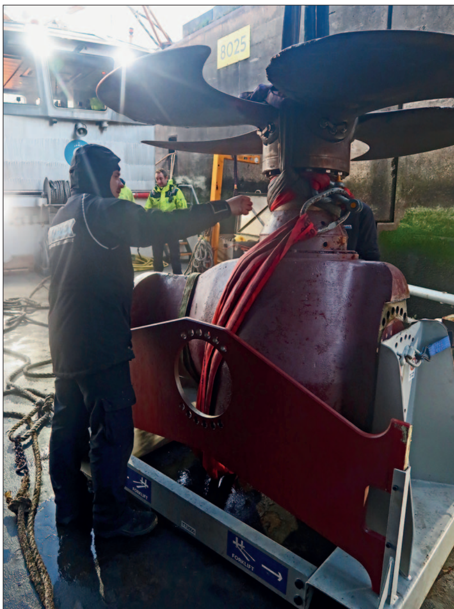
Hydrex diver/technician handling thruster unit during operation in Rotterdam.
