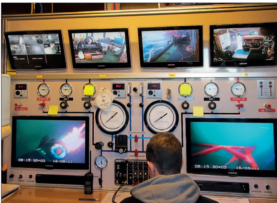
The dive station on board a workboat used to monitor dive operations during a major underwater repair.
