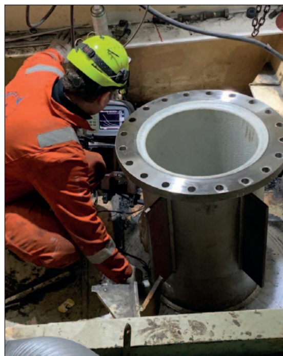
Independent non-destructive testing of the welds is always performed before the job is complete.
