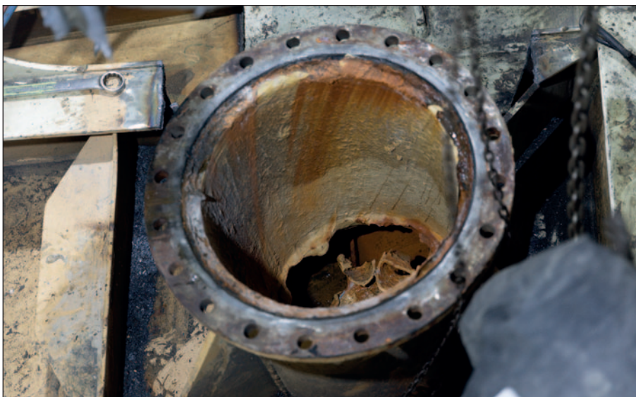
The old scrubber pipe seriously corroded by the highly acidic effluent from the scrubber.
