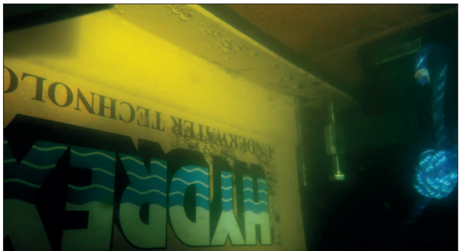
The cofferdam was positioned over the area where the transducer was to be installed.
