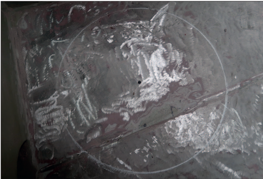
The shell plating was prepared for removal.
