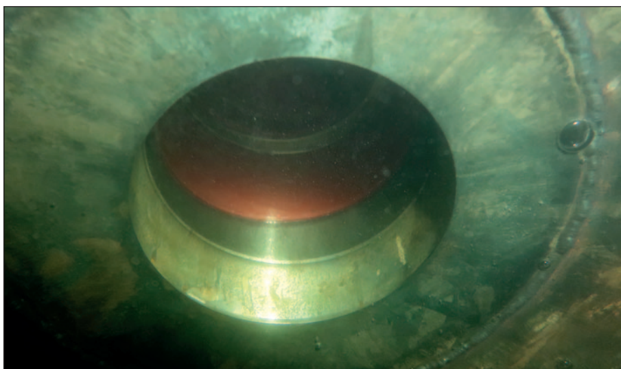
The new echo sounder flange seen from the outside.
