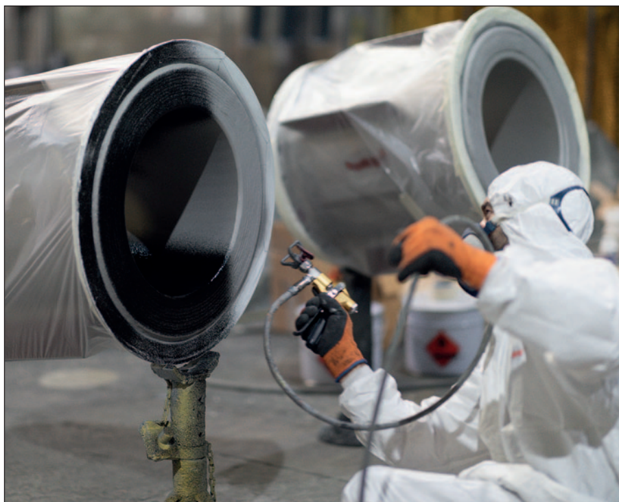
Scrubber overboard pipes receive proprietary protection with Ecospeed prior to installation.
