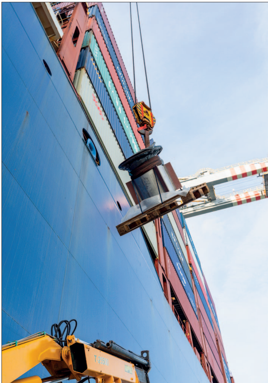
New overboard pipe lifted onto the ship.
