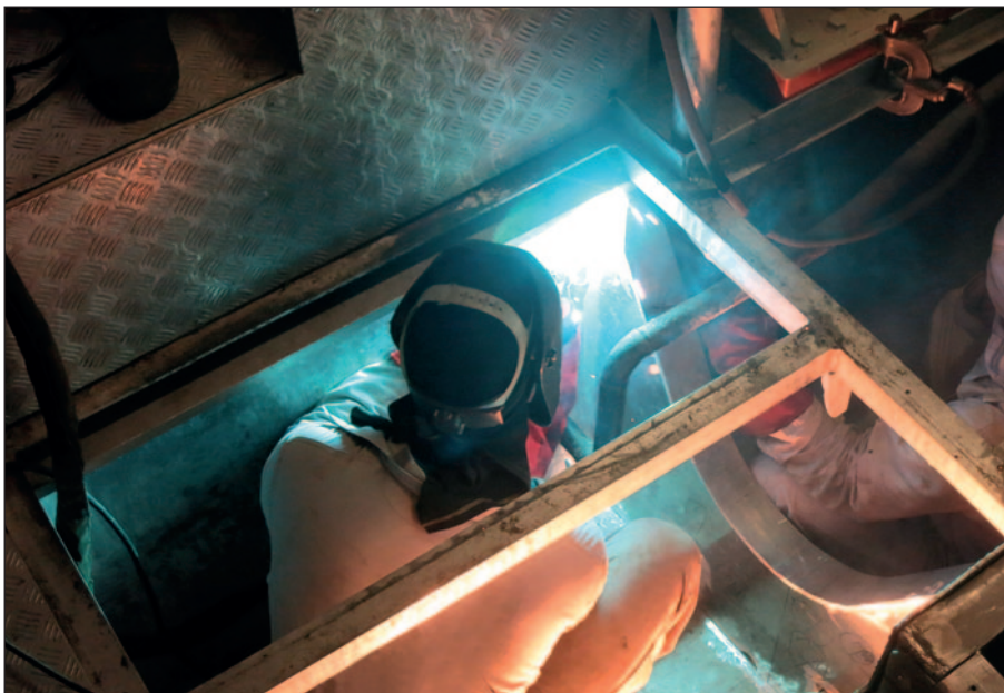
The shipyard needed to perform work on the shell plating from the inside while the vessel was afloat.
