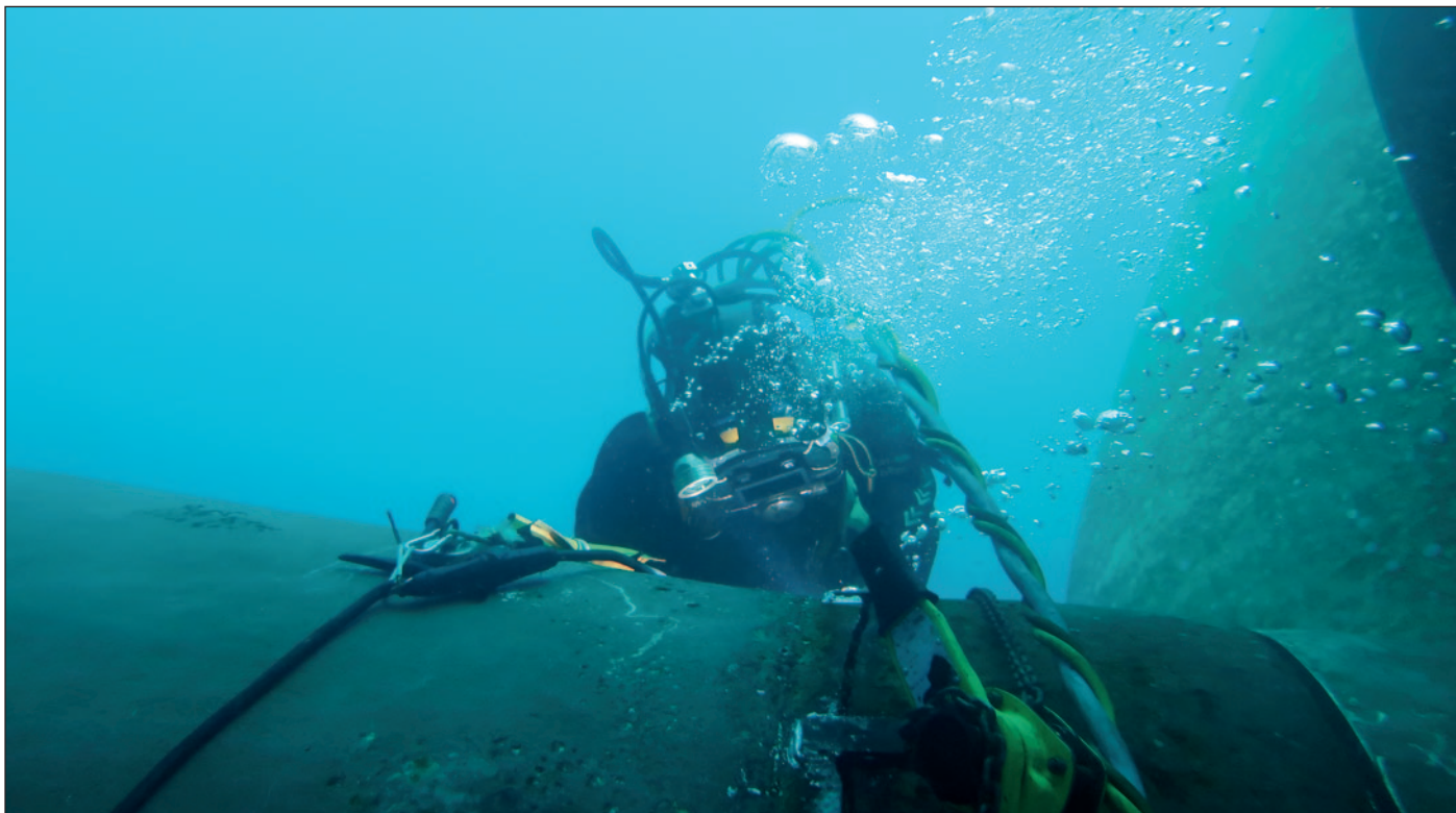
Hydrex diver working on the rope guard during stern tube seal operation.
