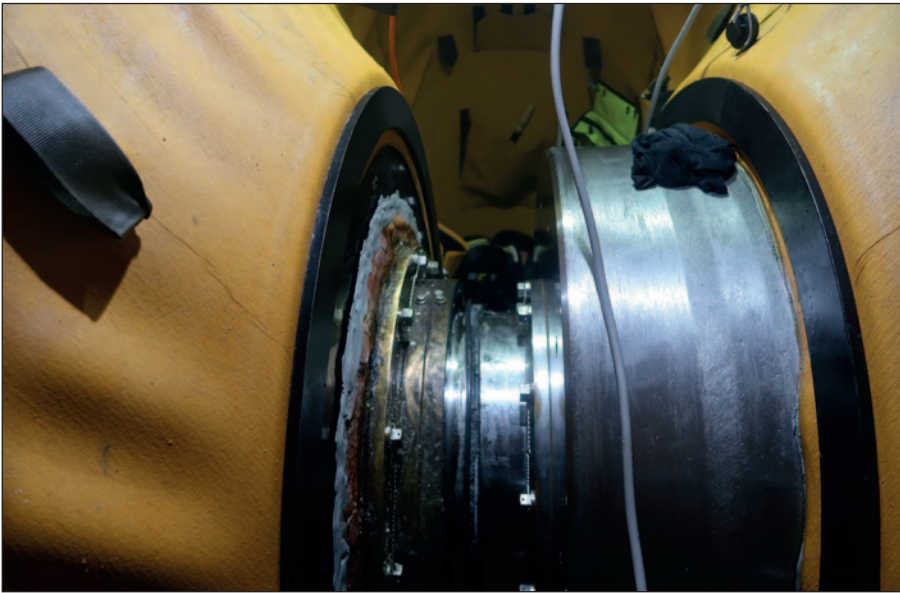
Stern tube seal assembly after mobdock installation.
