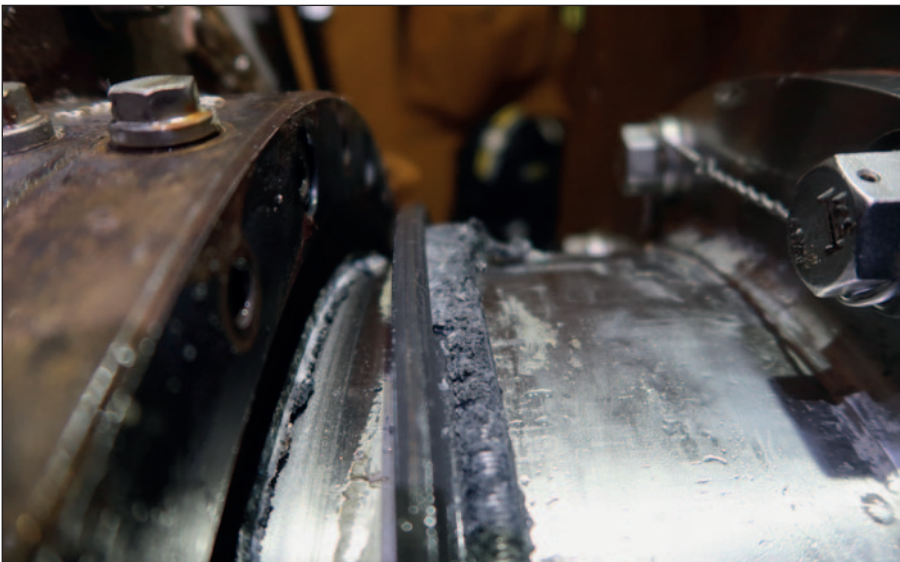
Damaged stern tube seal on general cargo vessel in Trinidad.
