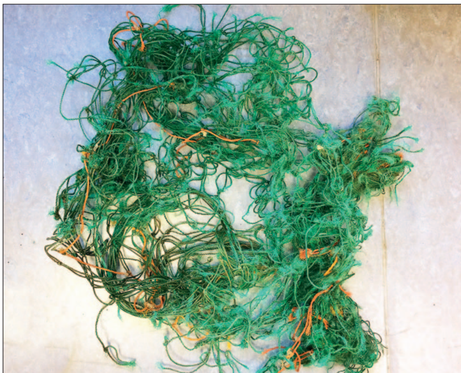
Netting removed from a ship's rope guard, found while on an inspection.
