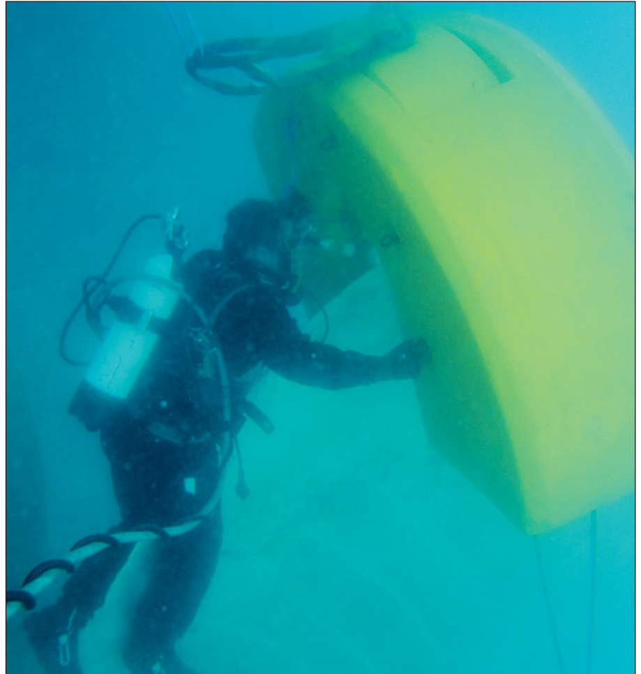
Hydrex diver positioning the cold straightening machine over one of the blades.
