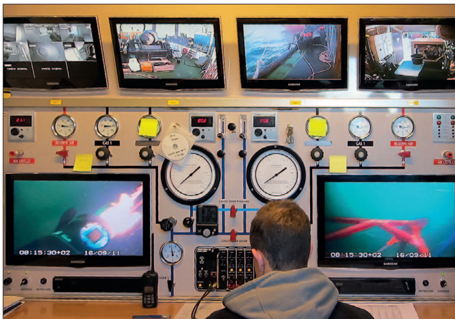
The dive station is used to monitor the work of the divers underwater, direct them as needed and record the operation.
