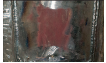
Class-approved underwater shell-plating replacement in Algeciras 4-6
