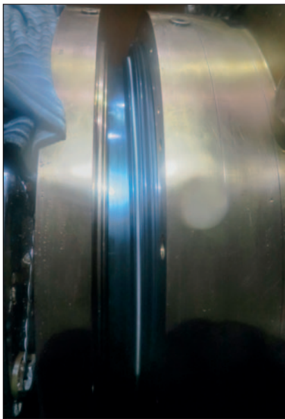
Successful seal repair leaves the stern tube as good as new with all leaks fully handled.
