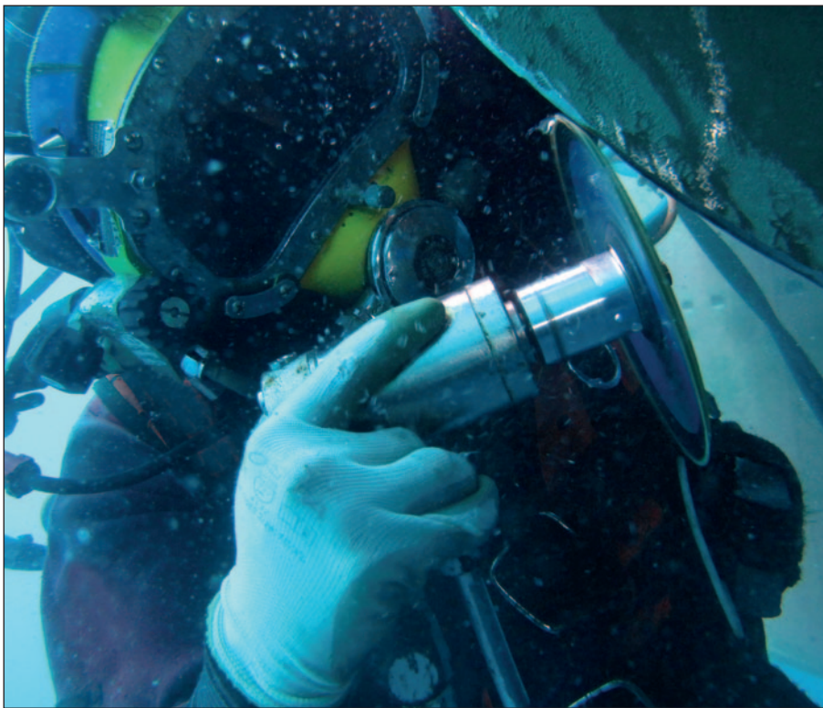
Hydrex diver carrying out grinding work on the trailing edge of one of the blades.
