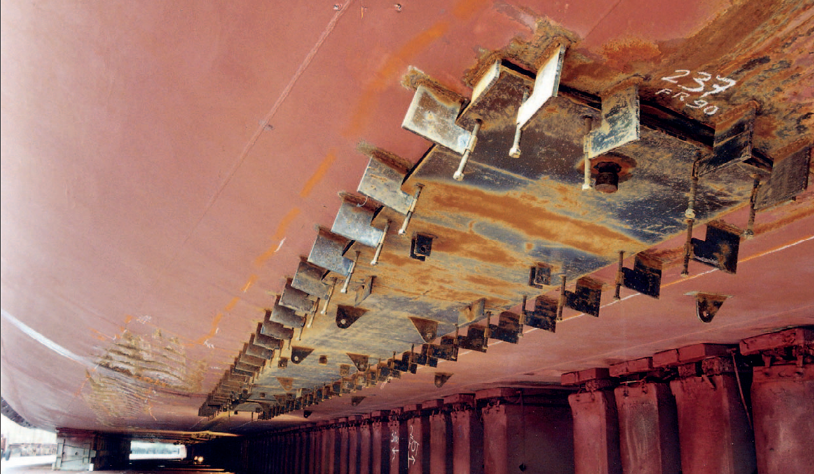
A ship successfully repaired after a severe grounding, now safely in drydock for permanent repair.
