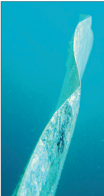
One of the five bent blades of a container vessel's propeller.
