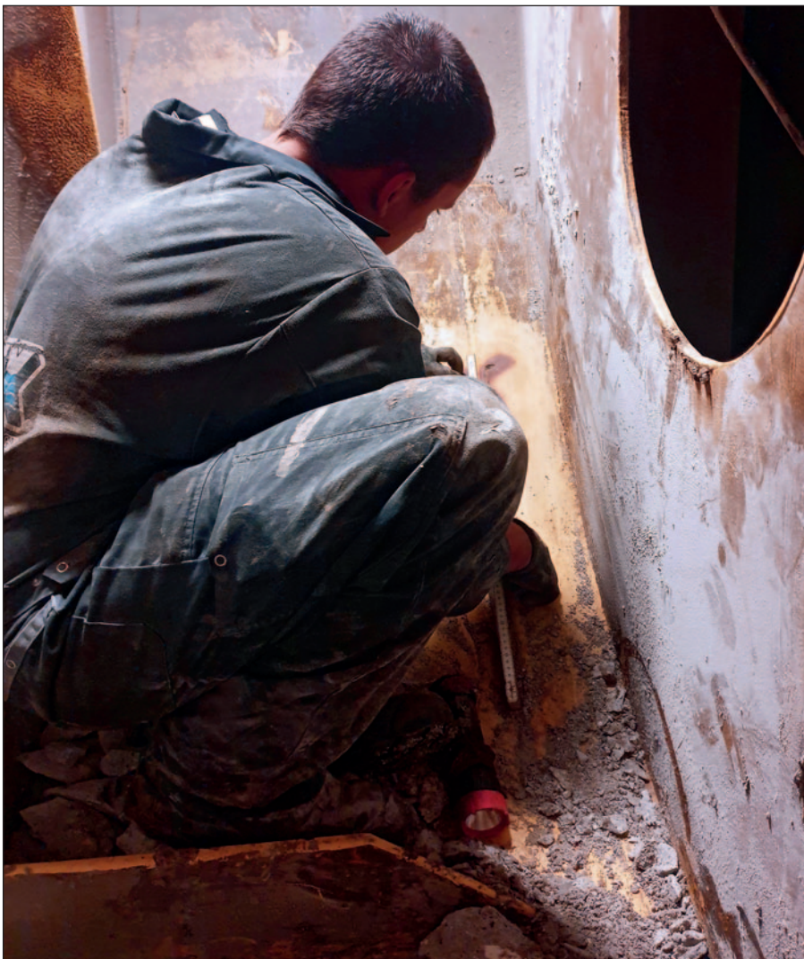
Hydrex diver/technician measuring the crack.
