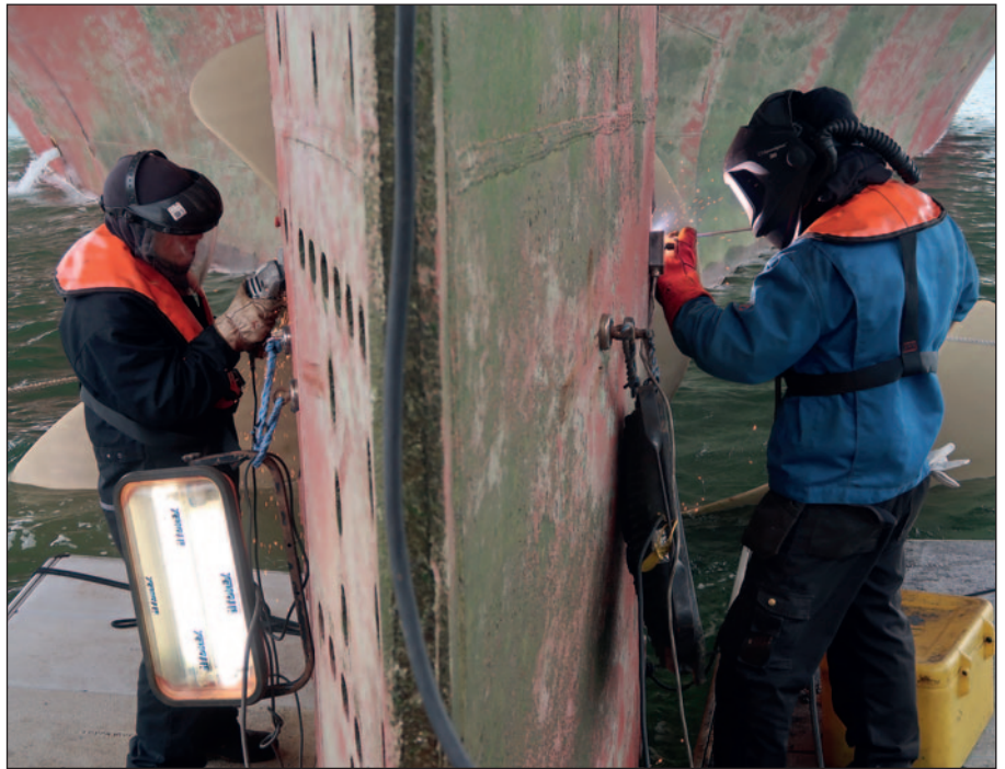
Hydrex diver/technicians repairing a rudder with the ship afloat, saving the costs and off-hire time associated with drydocking.
