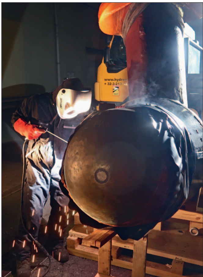
Hydrex welder welding the rope guards back in position on a thruster which has been removed for repair with the ship still afloat.
