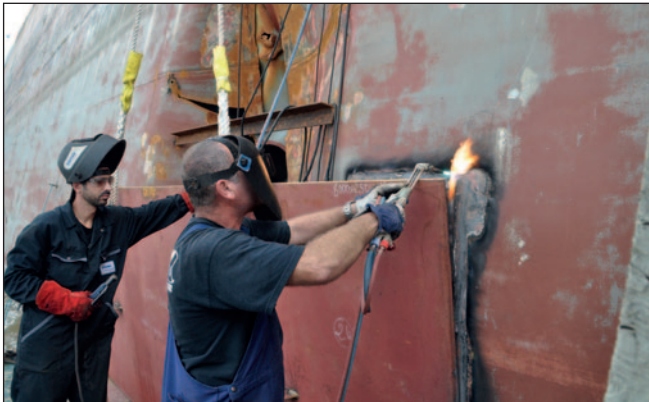
Hydrex team installing a large doubler plate on a bulker in Ivory Coast after collision.
