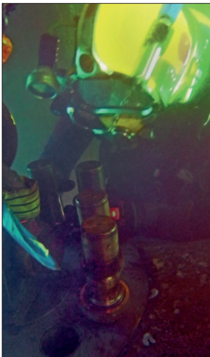
Bow thruster being prepared for removal in Italy a month before the reinstallation.
