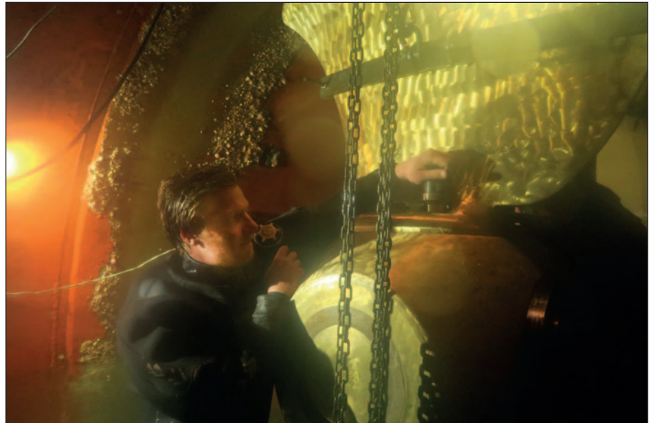
Installing one of the thruster blade bolts in Italy.
