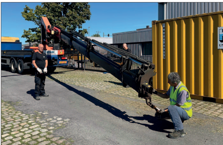
Inspection of lifting equipment by Daniel Bawin (right) of OCB, an independent testing and inspection company. Lifting gear is inspected every three months per Belgian regulations.
