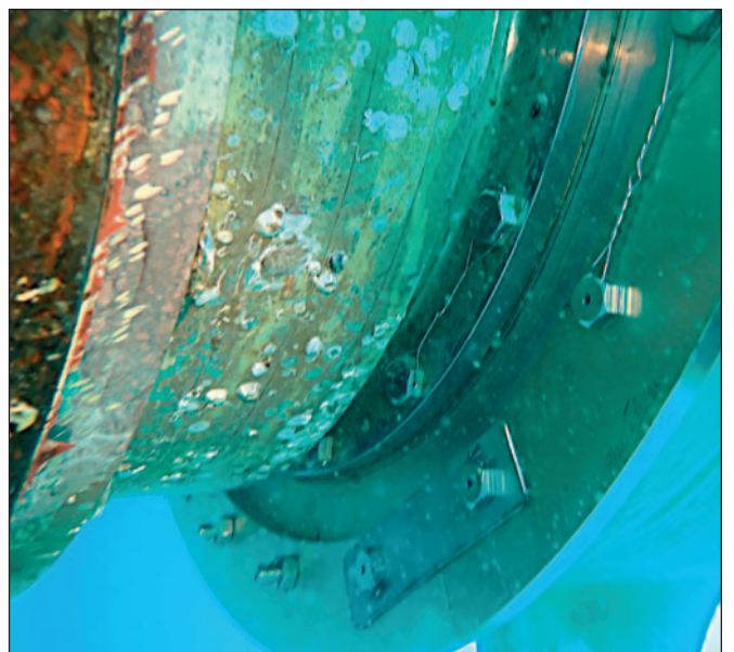
New split ring installed and secured.
