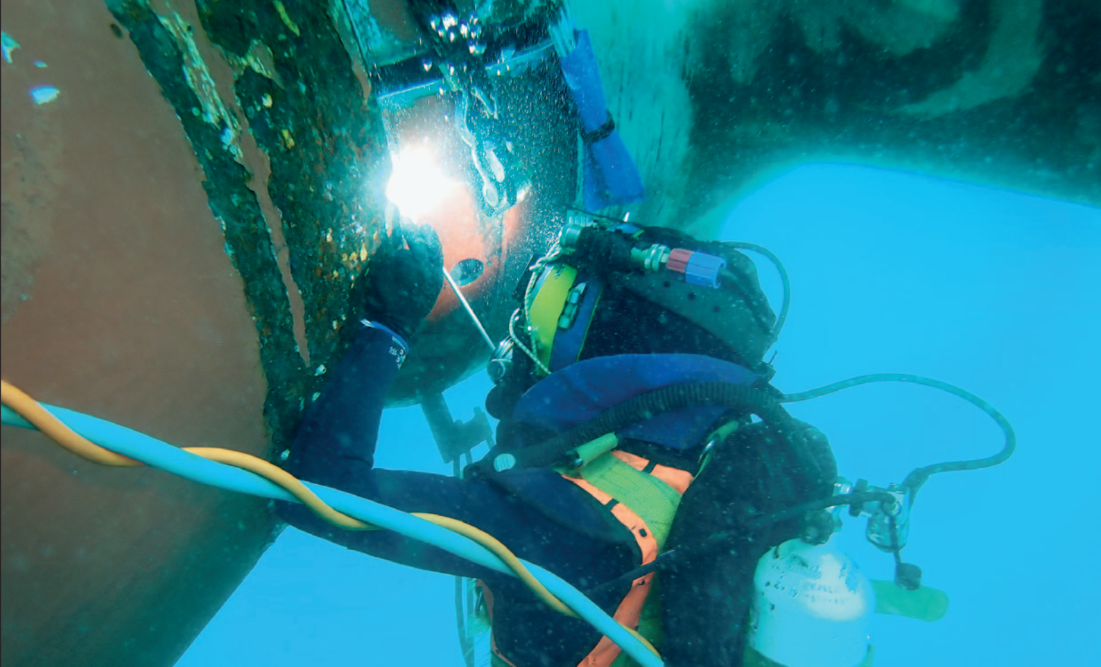
One of our diver/welders installing the new rope guard.
