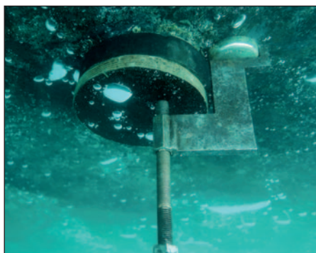
Depth sounder replacement by Hydrex divers.
