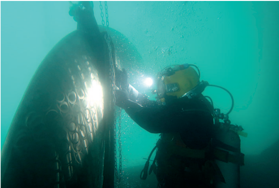
One of our divers guiding a new propeller blade during installation.
