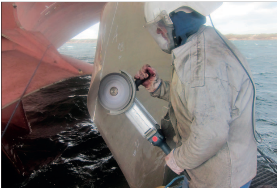
Both propeller blade straightening and cropping can be done underwater or on a trimmed vessel.
