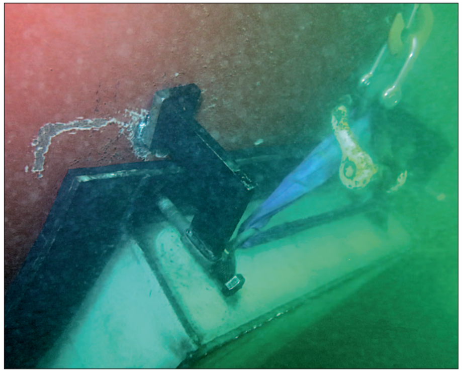
Cofferdam installed over crack on 360-meter bulker.
