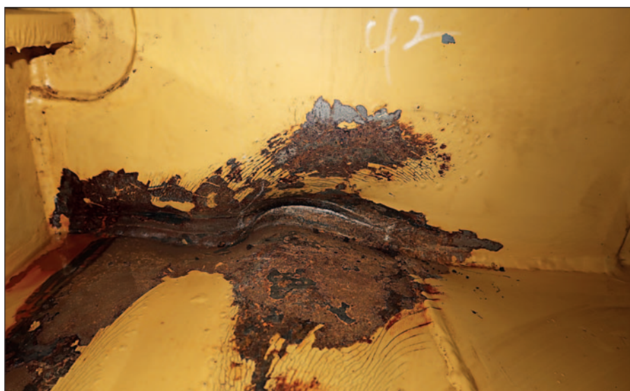
Crack in bottom plating after grounding.
