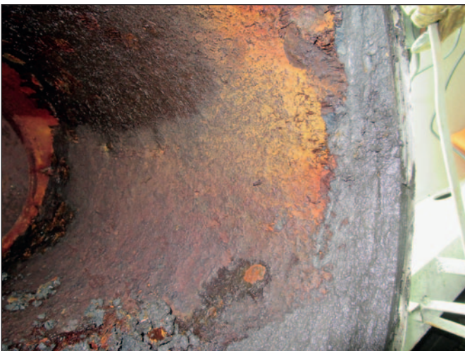
Corroded scrubber pipe seen from the onboard side.
