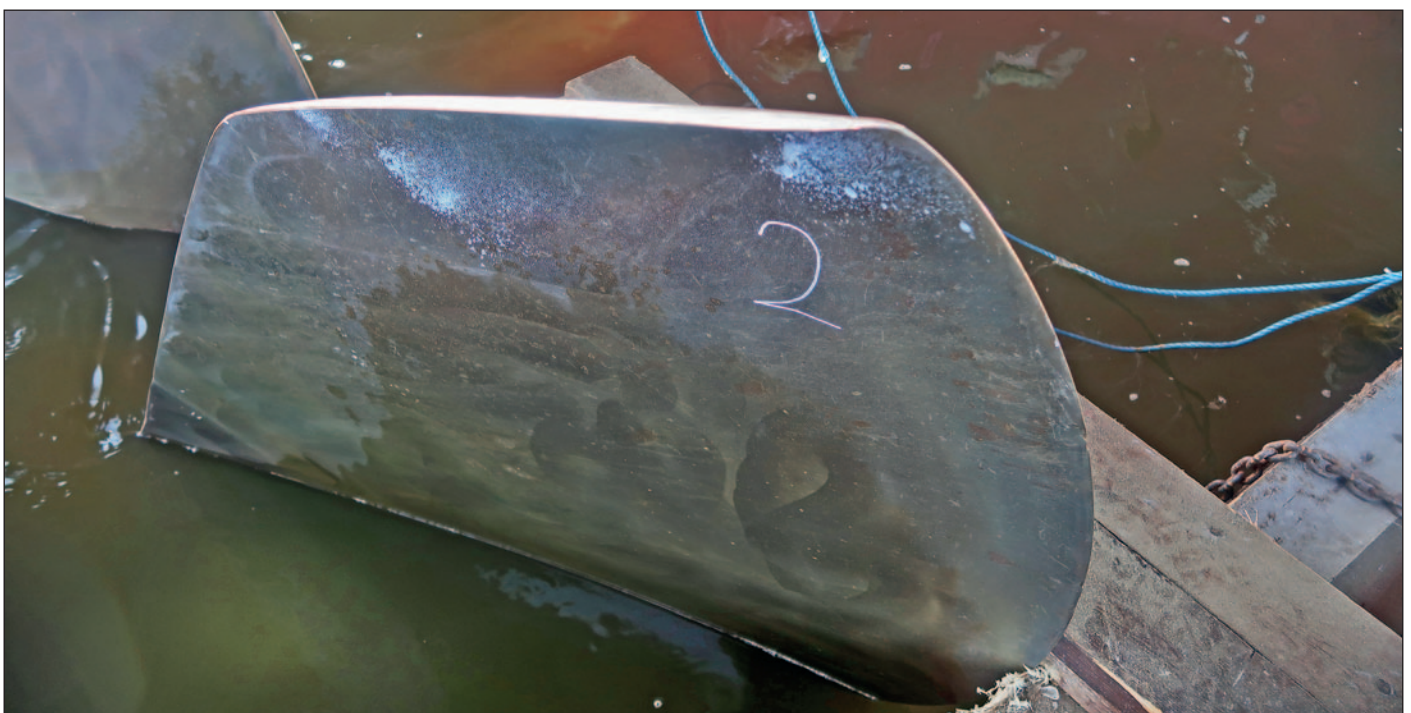
One of the cropped blades after grinding the edges. This is done for maximum efficiency.
