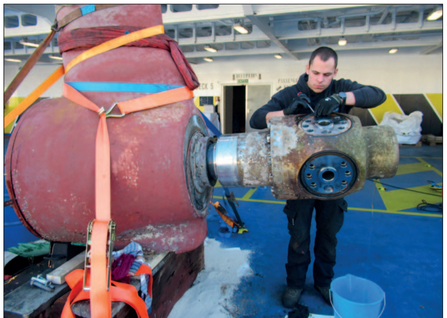
Hydrex technician during overhaul of the thruster.
