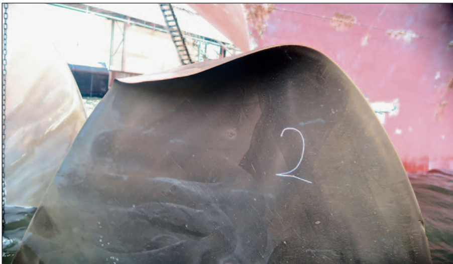
One of the five bent propeller blades of the bulker.
