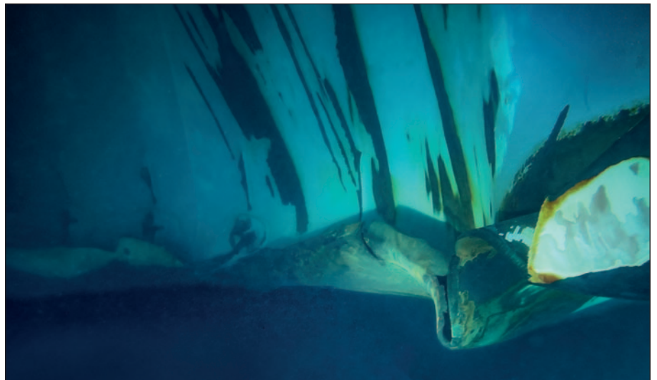
Severe damage to the hull from the grounding.
