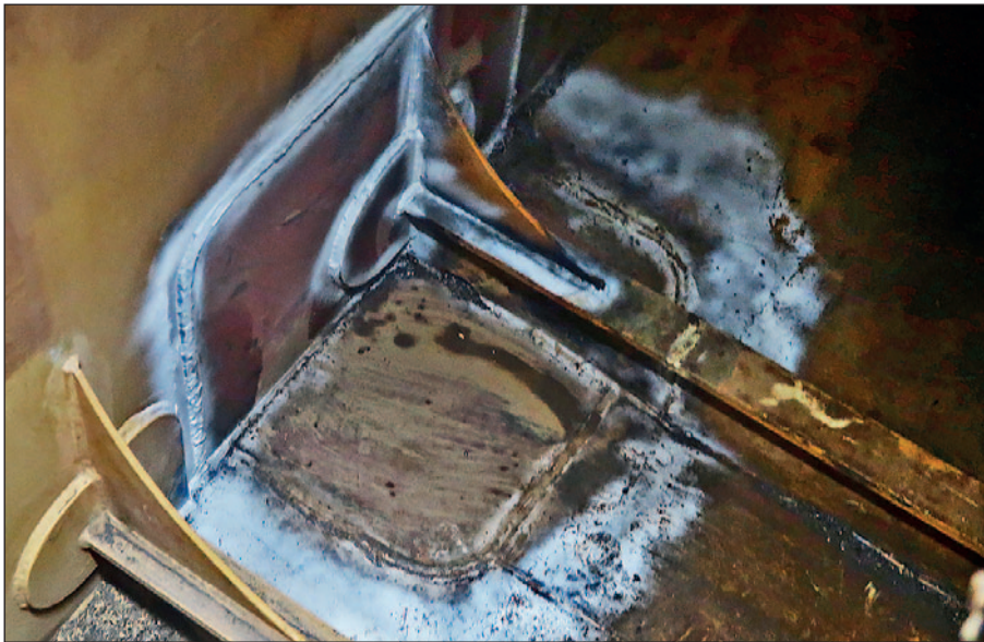
Completed insert repair with frames, brackets and split hopper plate repositioned.
