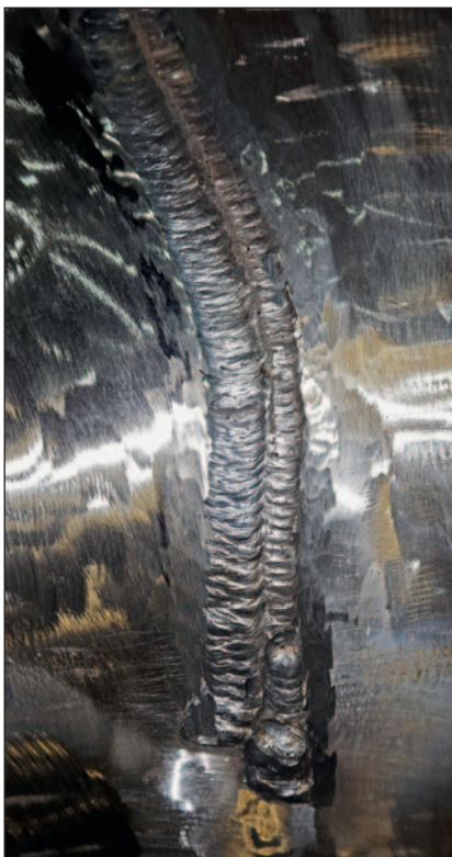
The crack after being filled up with a full penetration weld.
