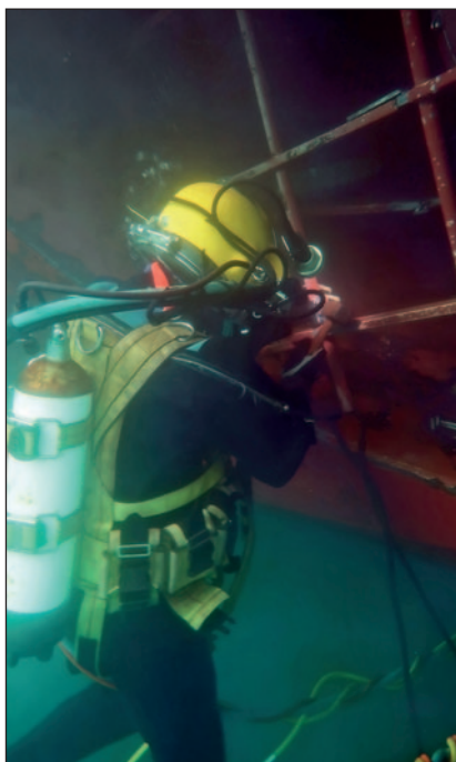
Hydrex diver working on the tunnel grids.
