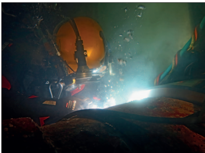
Welding work on the rope guard in Trinidad and Tobago.
