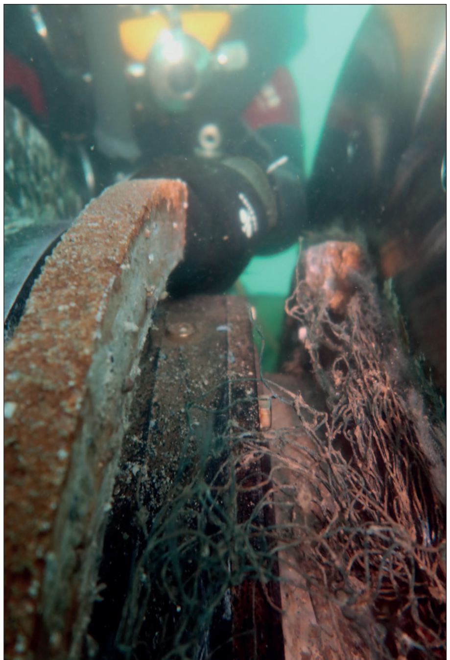
Diver removing fishing net caught in seal assembly.
