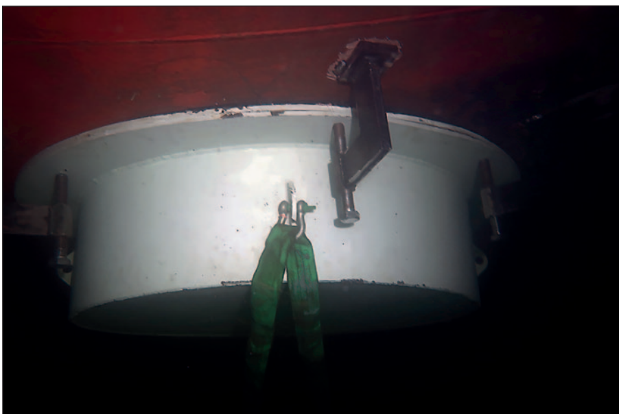
Cofferdam installed over the outlet of one of the scrubber pipes.
