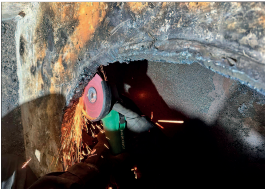
Preparing the edge of the shell plating for a new scrubber pipe.
