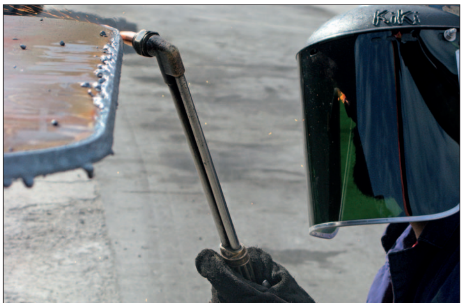
Hydrex welder preparing the insert plate in Palm Beach.
