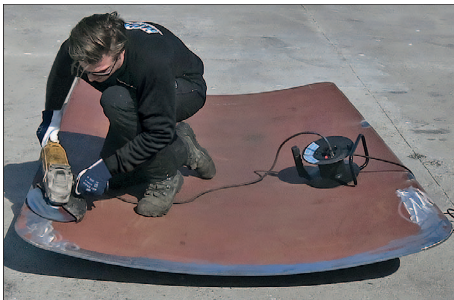
Preparing one of the doubler plates for installation in Las Palmas.
