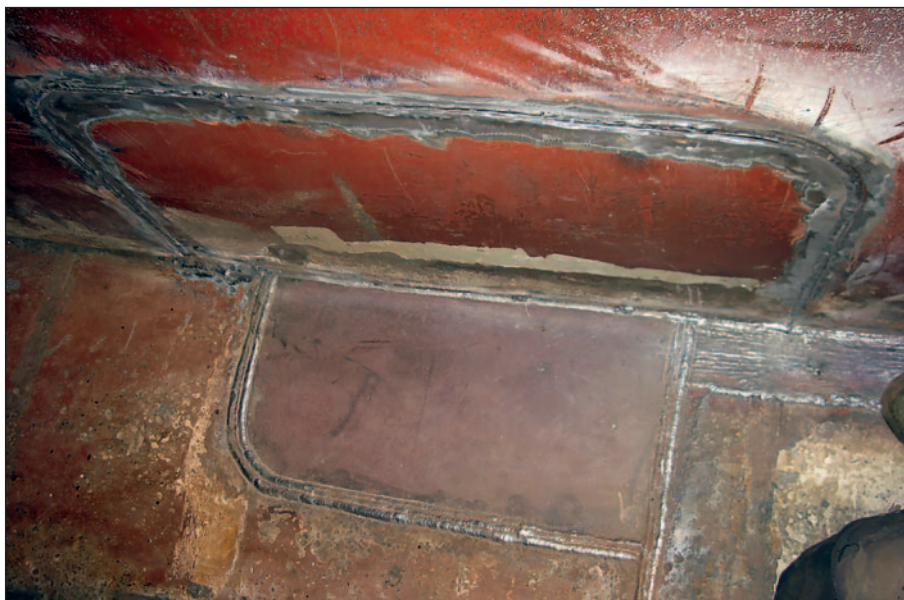
Finished insert with reinstalled frame.
