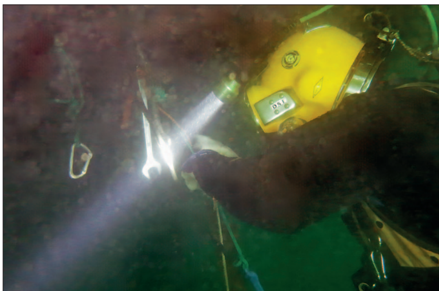
Hydrex diver/technician preparing the hull for installation of doubler plate.
