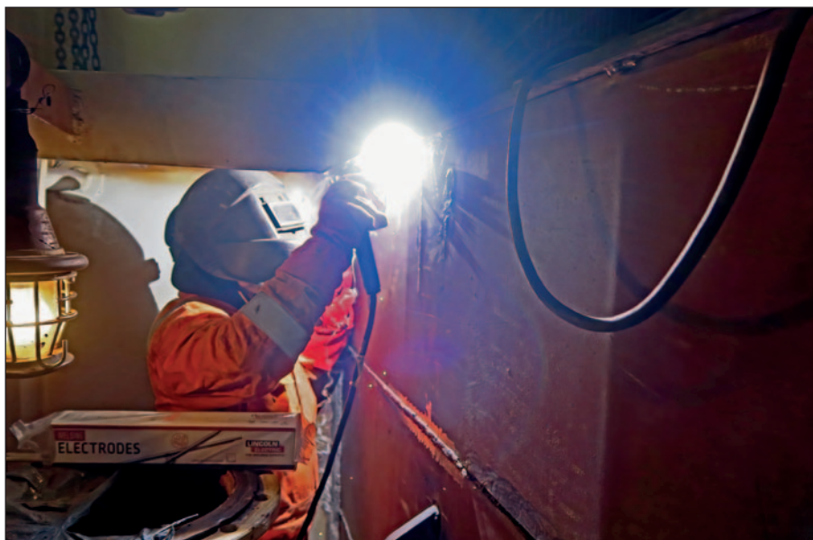
Securing the new inserts in Rotterdam with full penetration weld.
