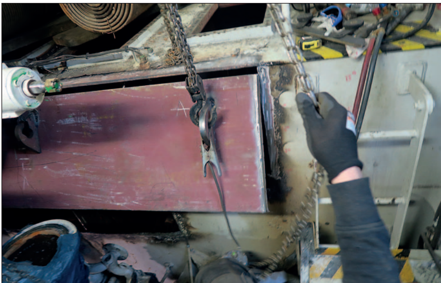
Positioning one of the new sea chest inserts.
