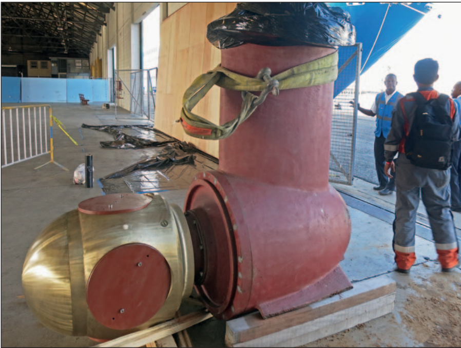
New bow thruster unit arriving on-site.
