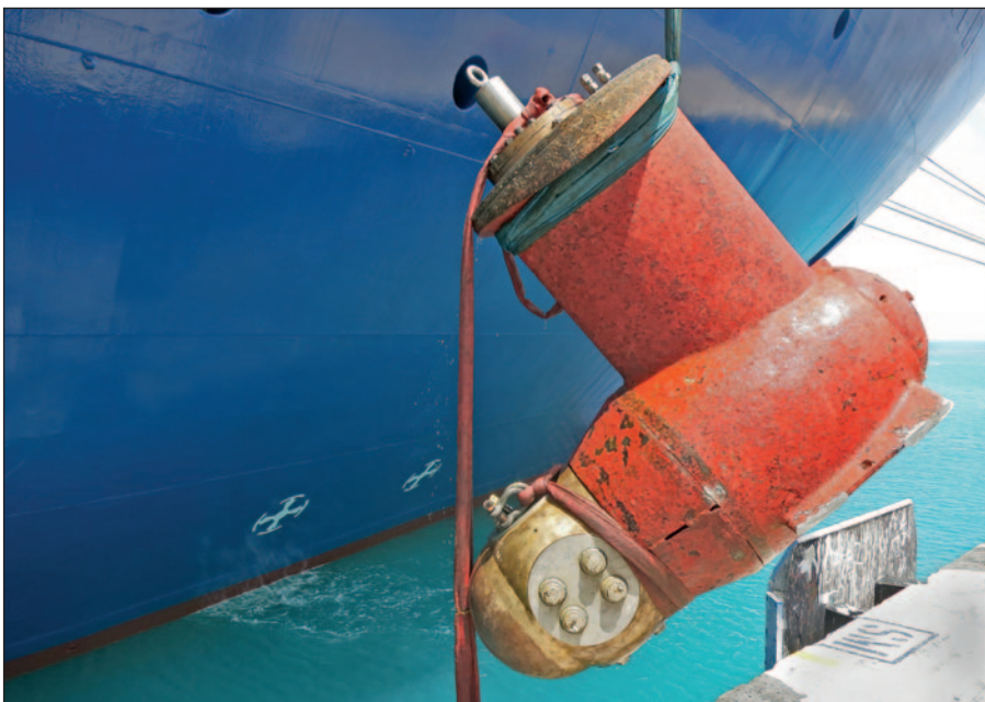
Old thruster unit brought to shore.
