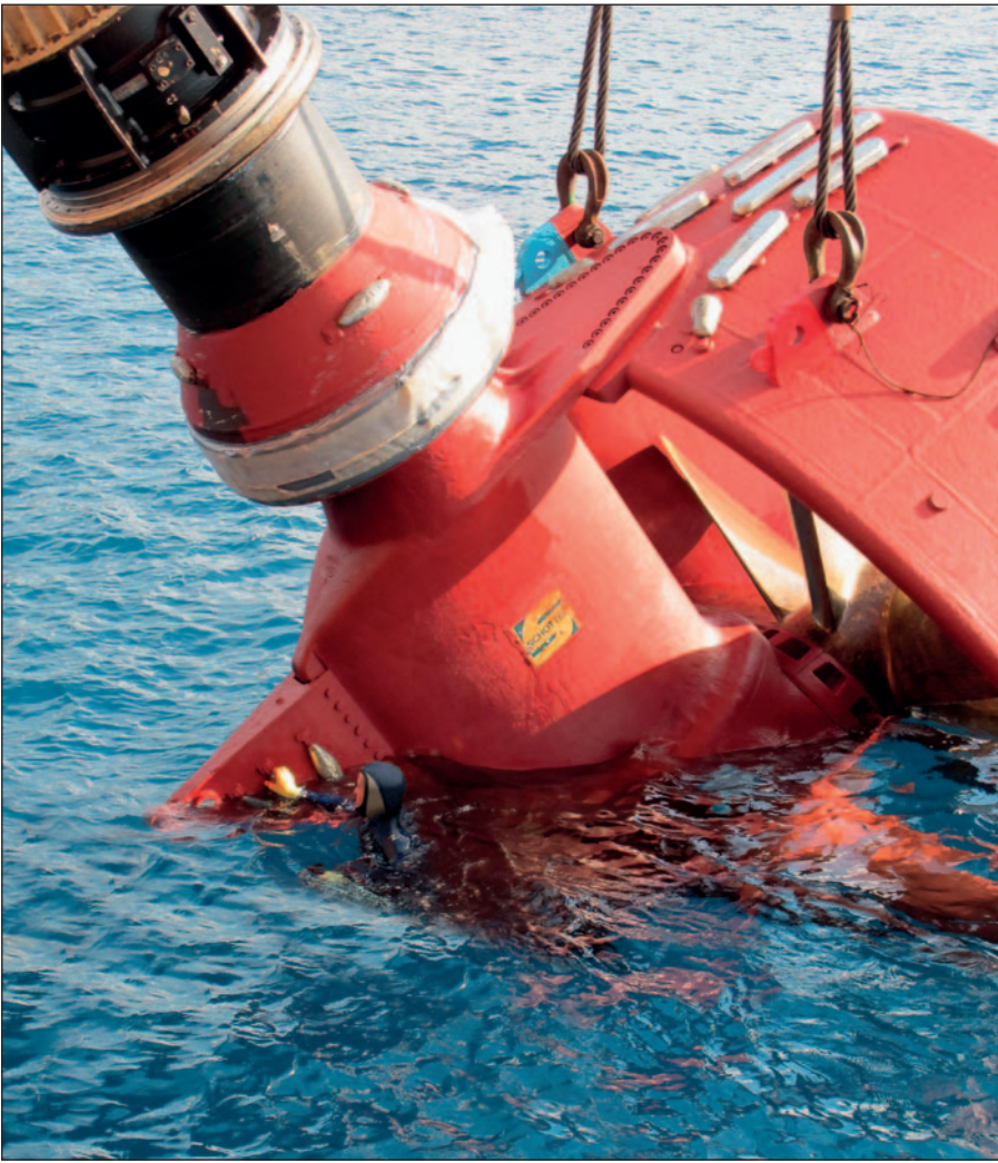
Overhauled thruster lowered back into the water.
