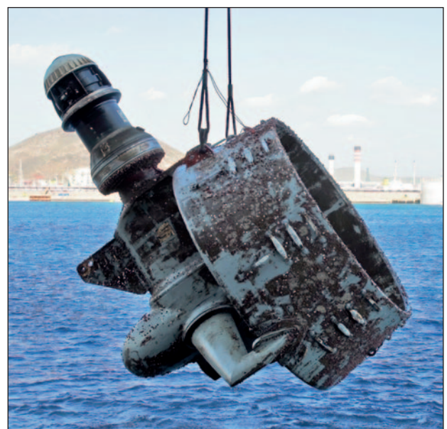
Azimuth thruster being lifted out of the water prior to overhaul.
