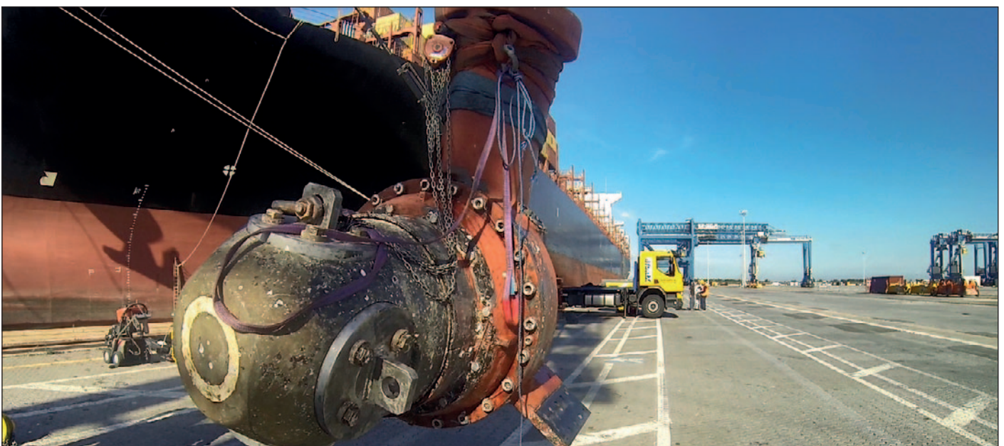
Bow thruster in Italy ready for overhaul after removal by our team.
