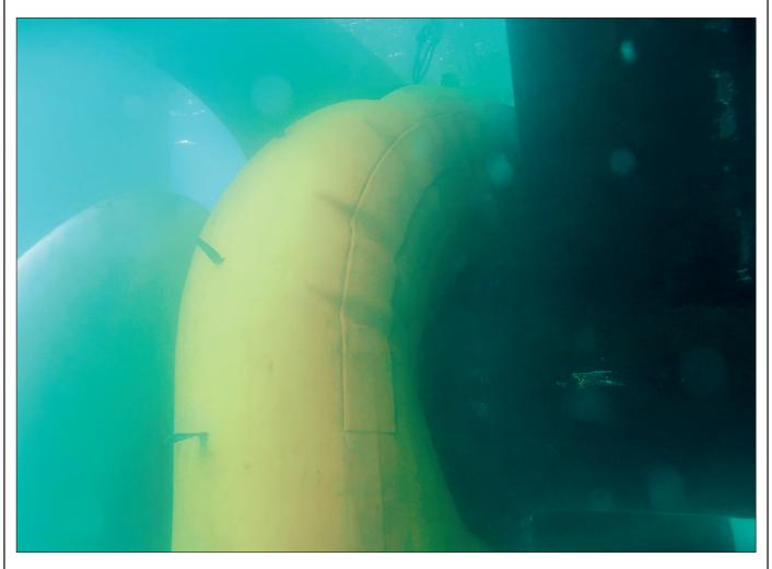
Using our flexible mobdock method to create a dry underwater environment, we have carried out stern tube seal repairs and replacements underwater for some years now in cooperation with OEMs.
