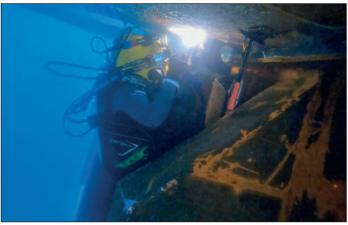
In 2022 a 45-ton cofferdam was designed to repair a large bulk carrier after a severe grounding.
