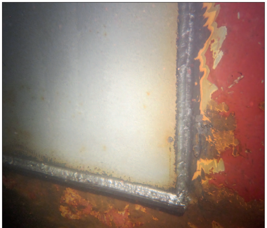
Weld seams of doubler plate installed over damaged hull area.
