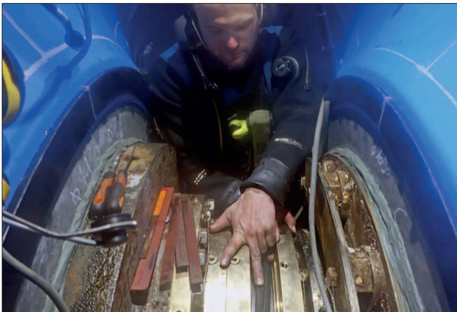
Two mobdocks were installed at the same time to work on both assemblies simultaneously.
