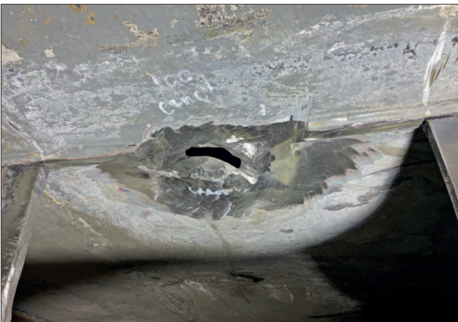
Crack on car carrier after being ground out.
