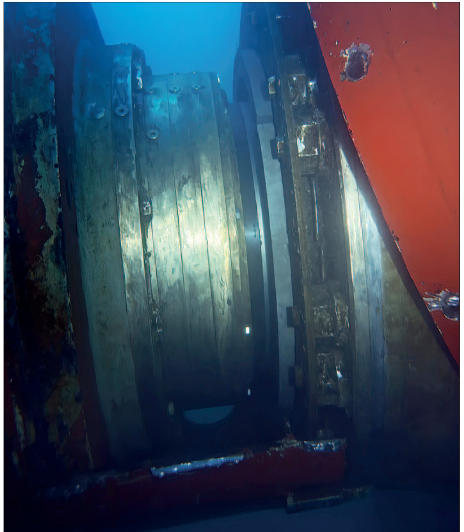
One of the seal assemblies after removal of the rope guard, prior to the repair.
