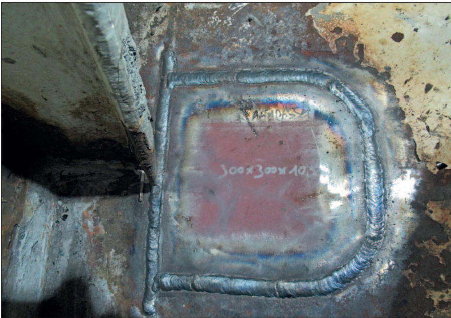
New insert installed on tanker in the Netherlands.
