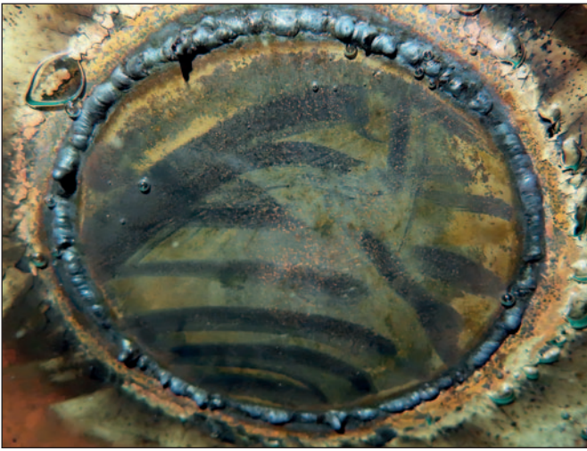
Insert with full penetration weld seen from the water side.
