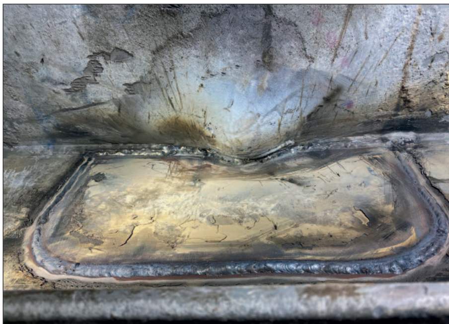
Crack repair after reinstallation of the longitudinal frame.
