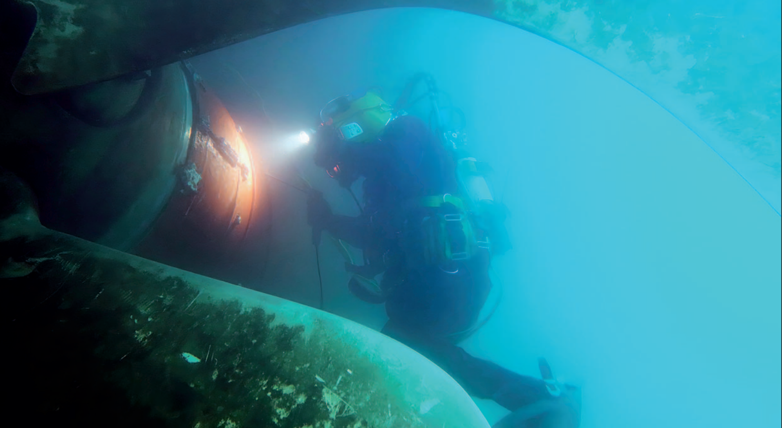
One of our divers during reinstallation of the first rope guard.
