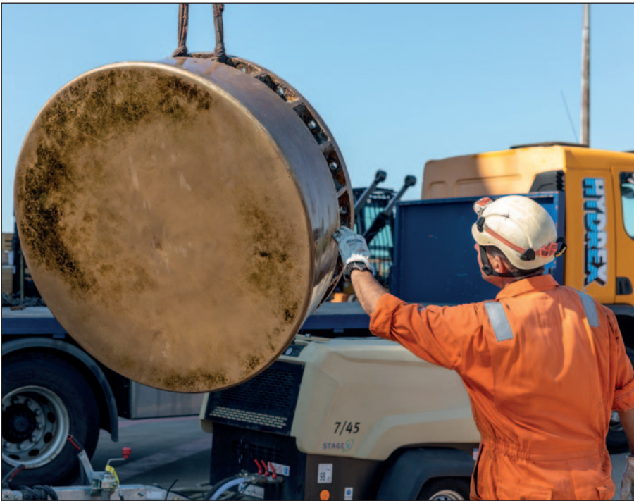
Old propeller cap lifted onto the quay side.
