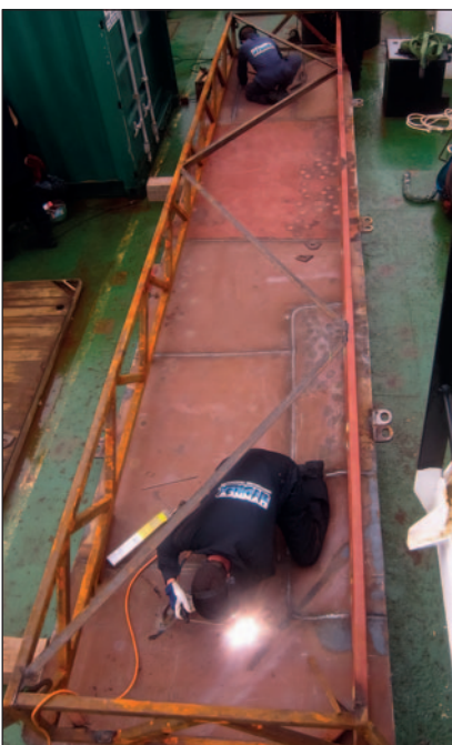
Preparing and lowering the doubler plate into the water so that it could be welded in place to repair the 8 x 1.8 m rip in the hull near the forepeak of the Navios Sagittarius.
