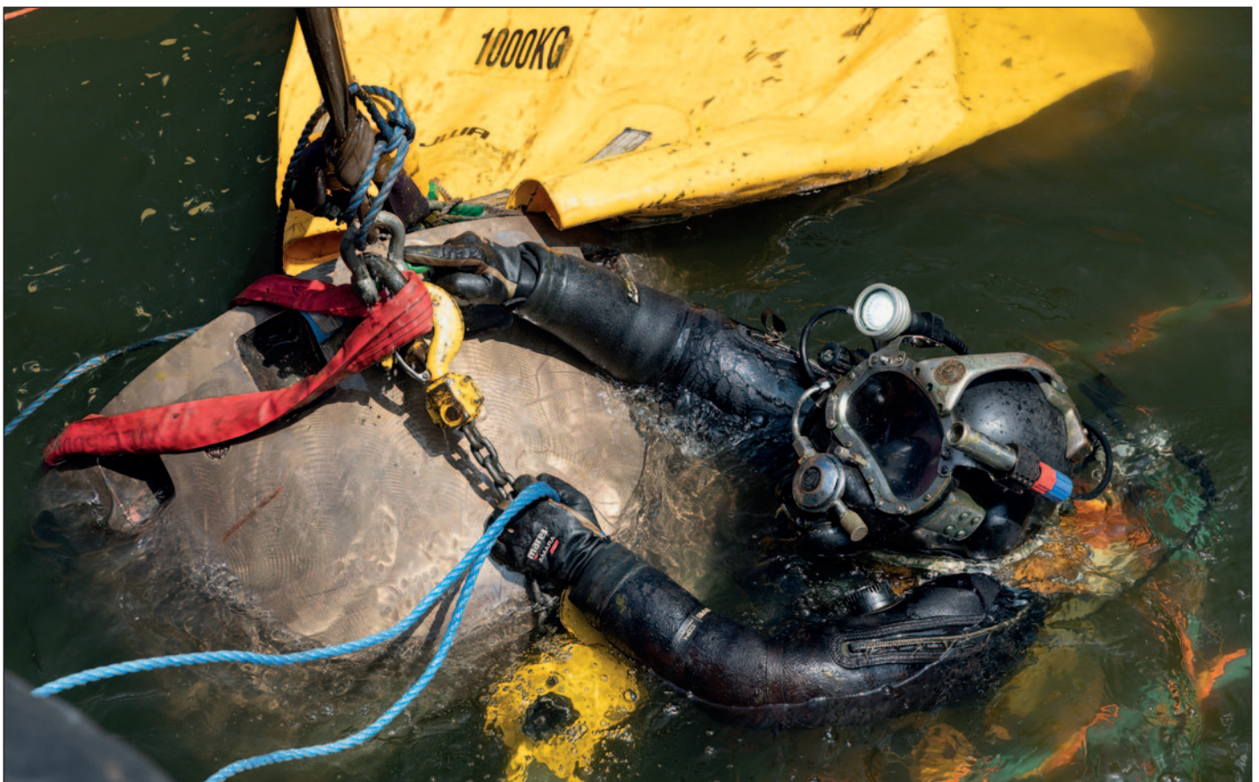
Hydrex diver during removal of the old propeller cap.
