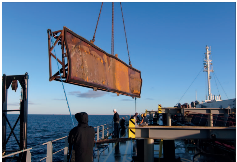
Preparing and lowering the doubler plate into the water so that it could be welded in place to repair the 8 x 1.8 m rip in the hull near the forepeak of the Navios Sagittarius.
