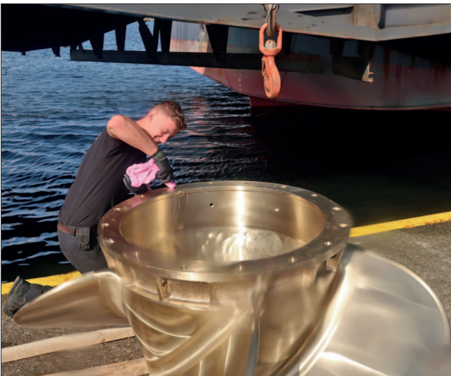
Final check of the propeller cone fin before installation.
