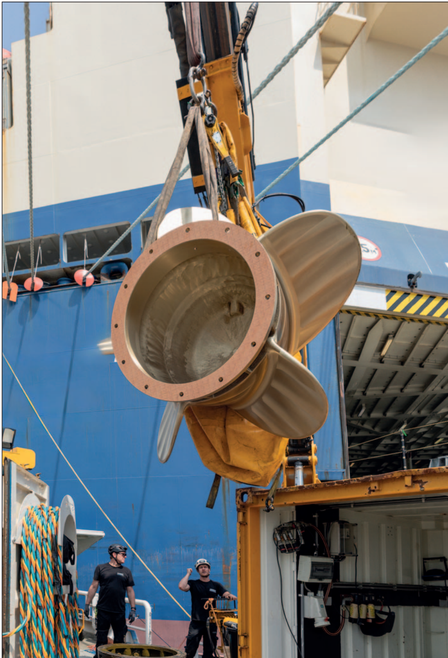
New propeller cone fin lifted with the crane of one of our workboats.
