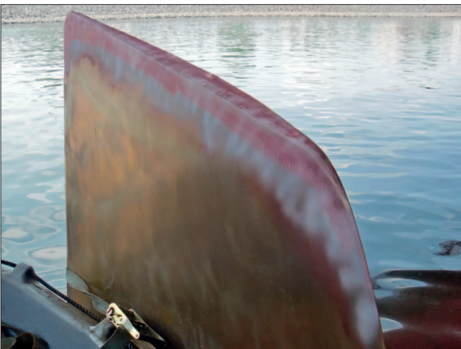
Testing one of the cropped blades for cracks.
