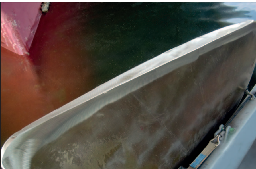
Cropped and polished propeller blade.
