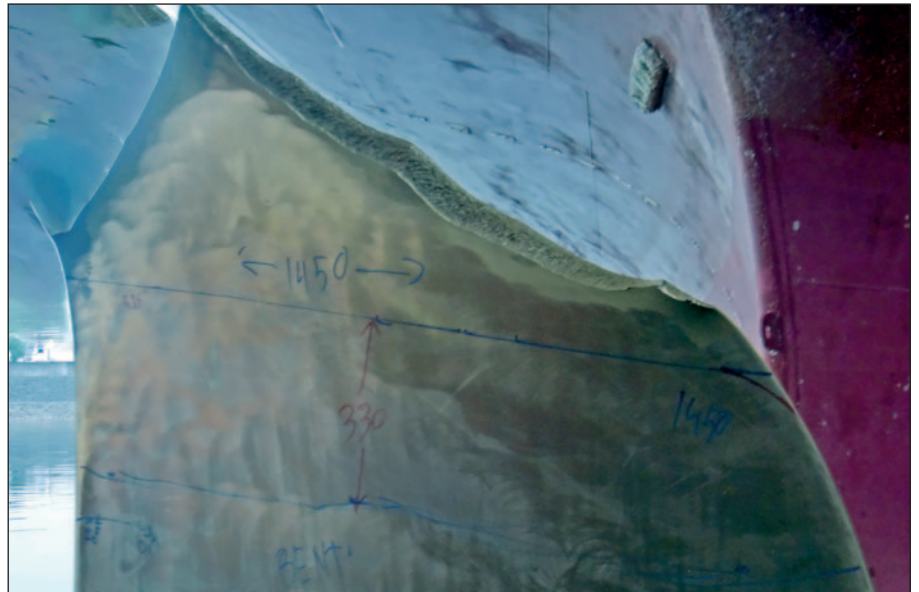
One of the propeller blades of a bulker was missing parts of its tip.
