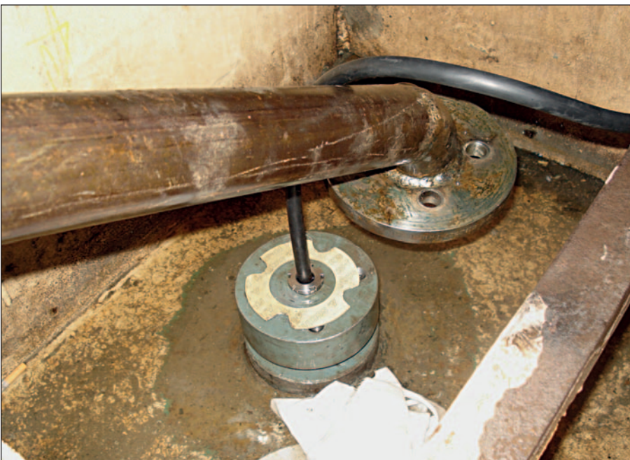
Any type of transducer can be installed or replaced afloat.
