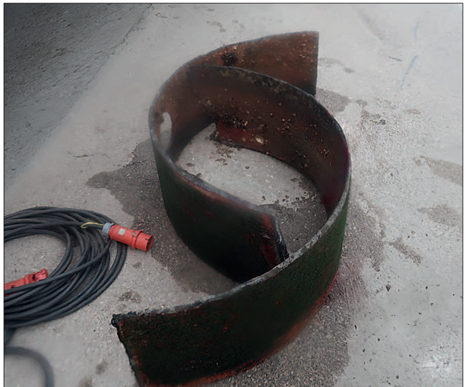
Rope guard of container vessel after removal.
