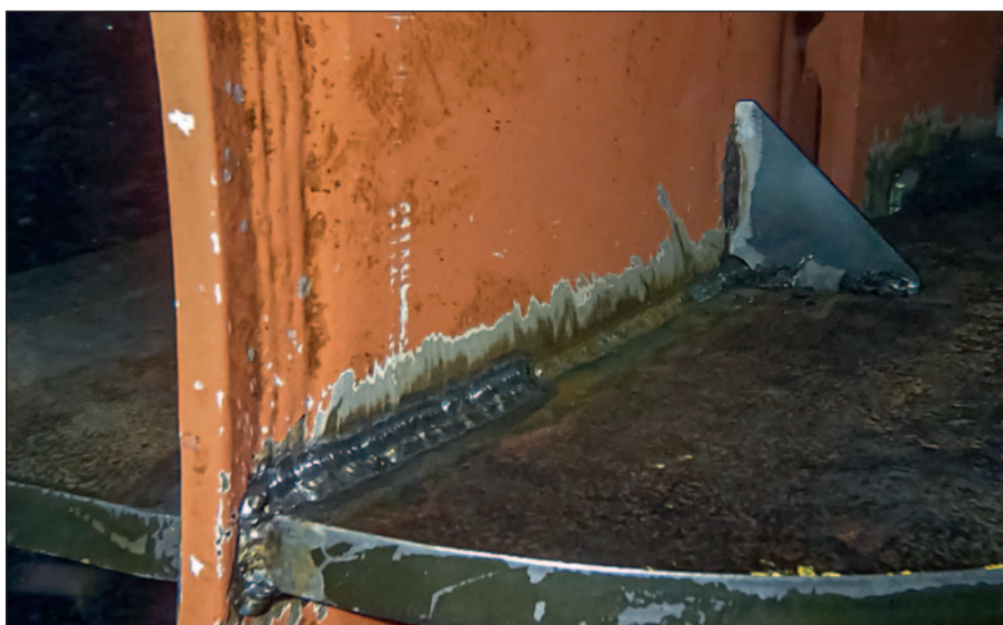
4 stiffeners were installed on each side of the rudder to secure the rudder flap.
