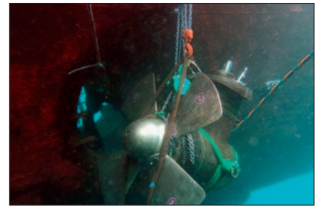
Bow thruster reinstallation in Algieras 7-9
