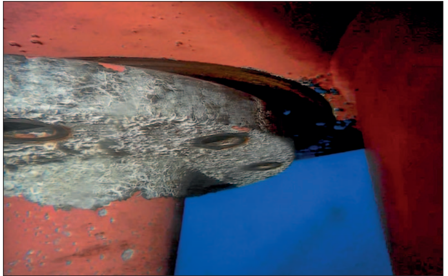
All bolts connecting the rudder flap to the rudder horn were broken off.
