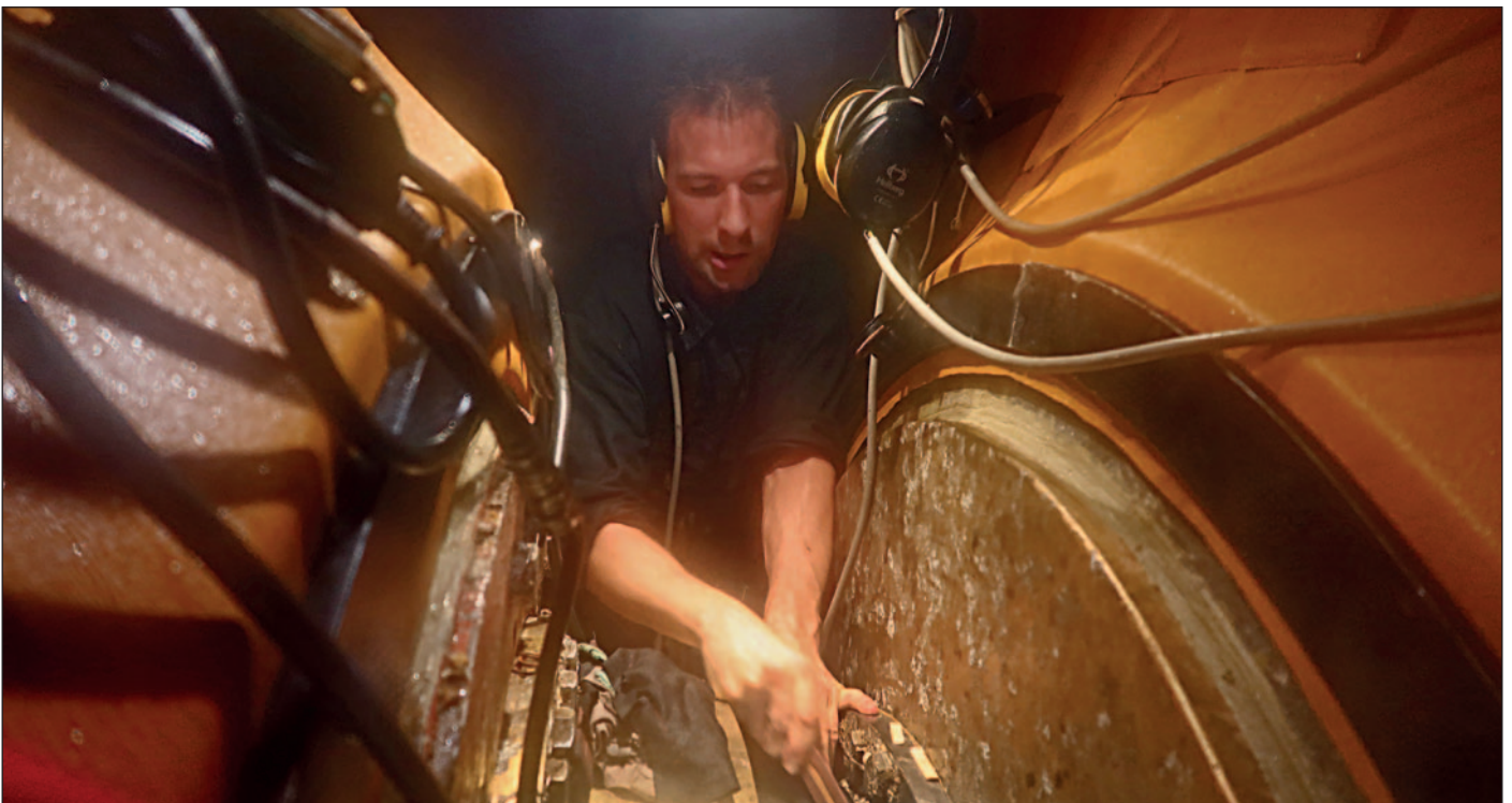
Hydrex diver installing the new stern tube seals.
