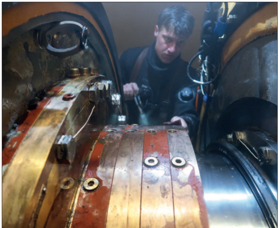
Hydrex diver working inside flexible mobdock in drydocklike conditions.
