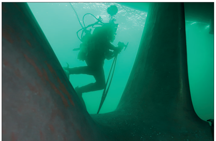
Hydrex diver getting ready to polish cropped propeller blade.
