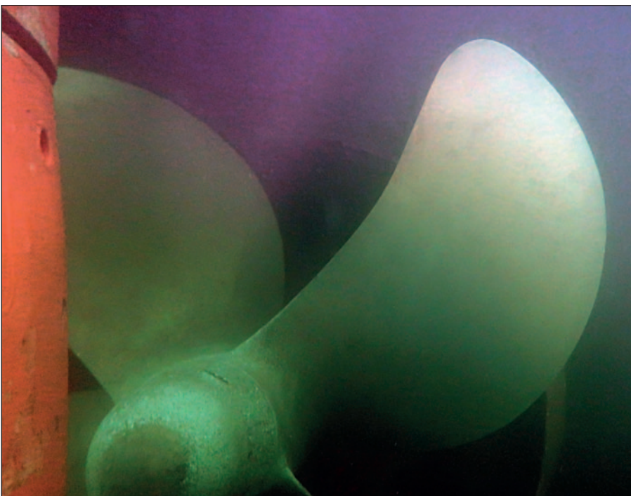
Propeller blade after straightening.
