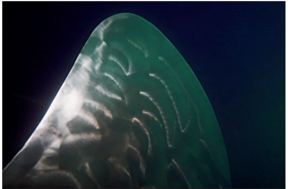
The blade was polished to restore its efficiency.
