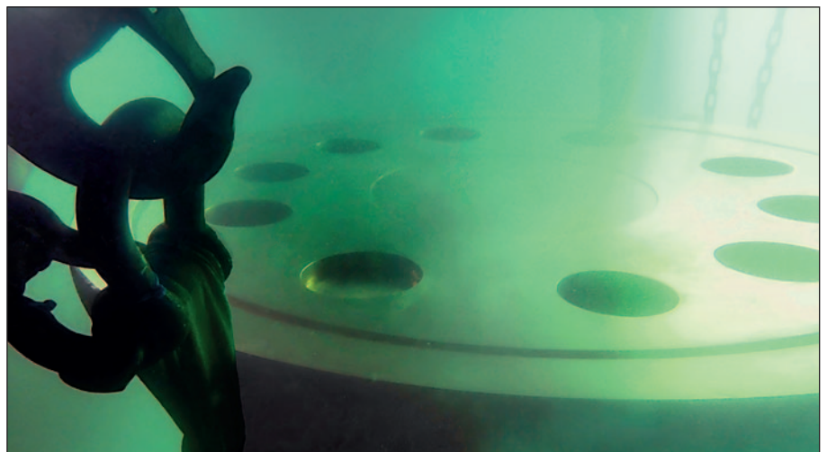
Propeller after removal of the leaking blade.
