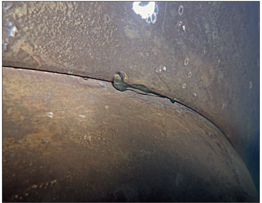
Oil was leaking from one of the propeller blades.
