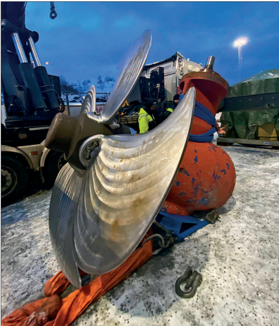
Old bow thruster after being brought to shore.
