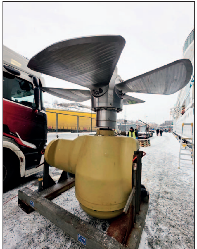
New bow thruster arriving on-site.
