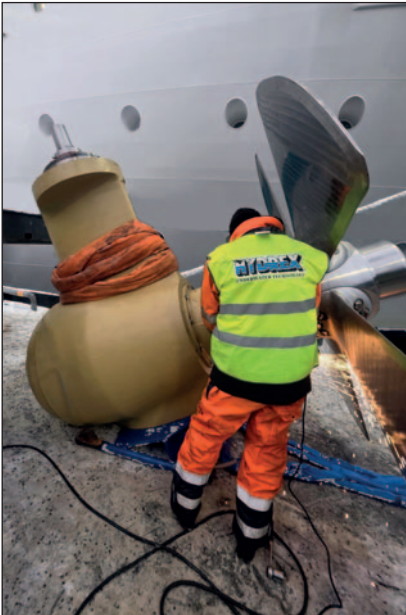
Preparing the new bow thruster for installation.
